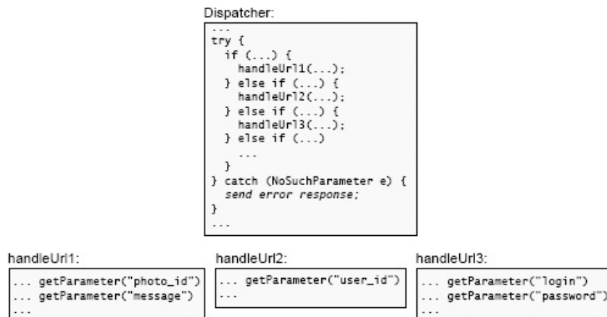
Figure 10.2: This code is functionally equivalent to Figure 10.1 , but exception handling has been aggregated: a single exception handler in the dispatcher catches all of the NoSuchParameter exceptions from all of the URL-specific methods.
